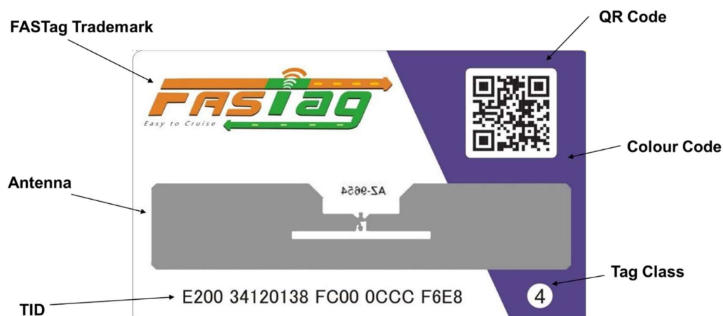
FIGURE 4 - FRONT- ADHESIVE SIDE OF NHAI FASTAG
