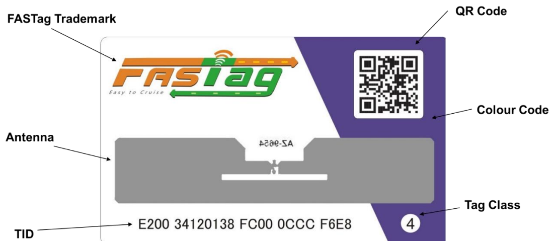
FIGURE 4 - FRONT– ADHESIVE SIDE OF NHAI FASTAG
