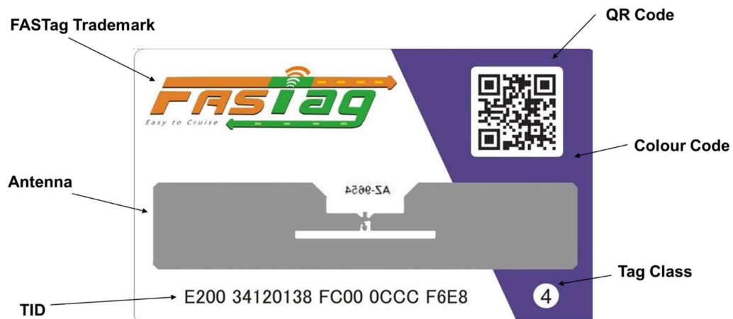
FIGURE 4 - FRONT- ADHESIVE SIDE OF IHMCL FASTAG
